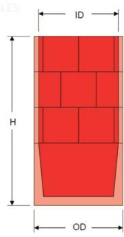
NOTE: Crucible assembly heights (H) can be changed to suit furnace sizing by adjusting side brick height and/or course count.
